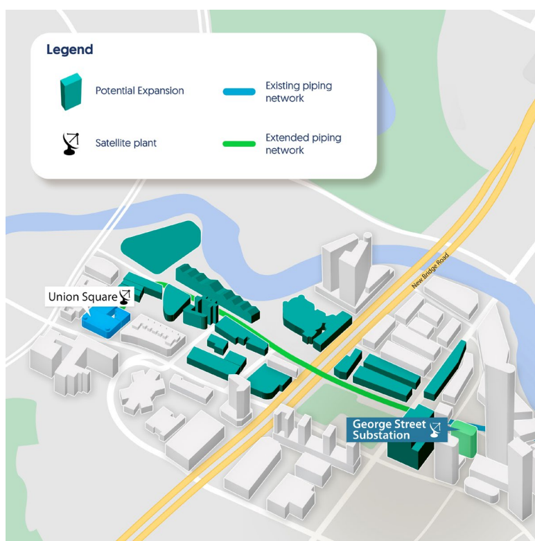
Union Square will house a District Cooling Satellite Plant connected to SP Group's district cooling network, serving its commercial components and future developments in the area. (Source: SP Group)
